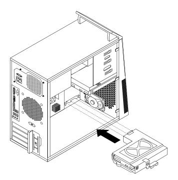
Figure 40. Installing the secondary hard disk drive
